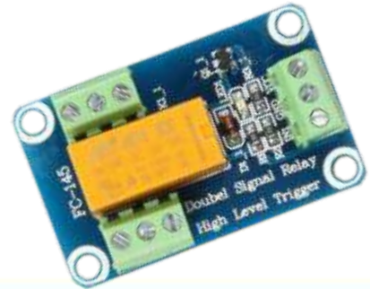
2 X 5V DC High Level Trigger Relay Module
