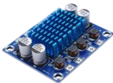
T1051 XH-A232 TPA3110 30W+30W 2.0 Channel Digital Stereo Audio Power Amplifier Board
