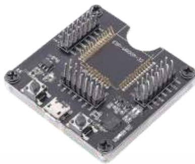
T1121 7Semi EC200U-CN LTE 4G GNSS Ultra-compact Nano Modem
