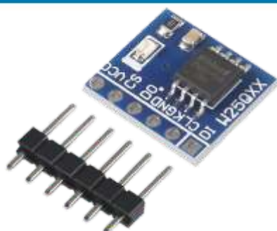
T1061 W25Q32 Large Capacity Flash Storage Module
