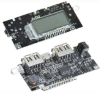
Dual USB 5V 1A 2.1A Power Bank Charging Module
