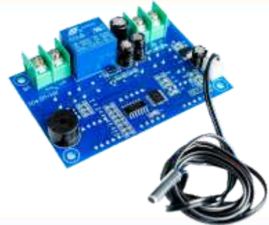
XH-W1401 DC12V Digital Thermostat Temperature Controller With NTC Sensor
