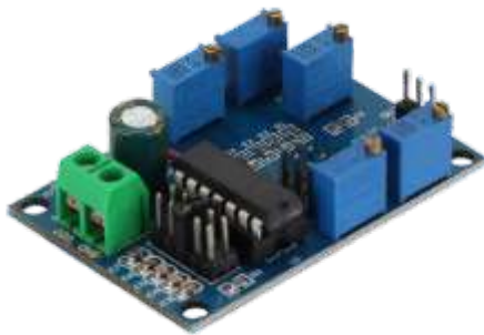
T1047 Triangular/Rectangular/Sine Wave Generator Module
