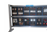
46609A Power Distribution Trainer
