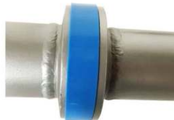
Hubs, O-Ring and locating ring assembled
