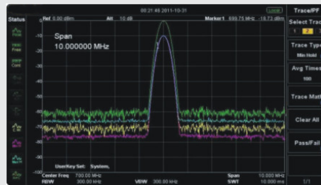
Compare the spectrums when change the RBW settings with different color trace
