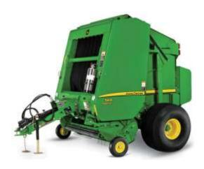
Height x width 36x46cm14x18in. Length 30.5 to 127 cm12 to 50 in. Pickup width 187.9 cm74 in. Tooth bars/teeth 6 bars, 156 teeth Lift control Crank (hydraulic opt.) Pickup diameter Compression rack rods 49.5 cm19.5 in.
