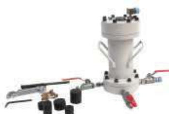
Triaxial Testing of Rocks
