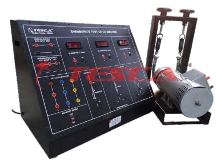
46602 Swinburnes Test of DC Machine is an important training system for Electrical Laboratories. It can be aptly employed for understanding the fundamental concepts and functioning of DC Motor. Swinburnes Test is the method through which losses are measured separately and efficiency at any desired load can be predetermined.
