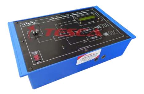
52005 Ultrasonic digital distance meter has been designed specifically for measuring distances between 0.2 meters to 4 meters. After Processing the data from the ultrasonic sensor the measuring distance is shown on a 16x2 alphanumeric LCD.
