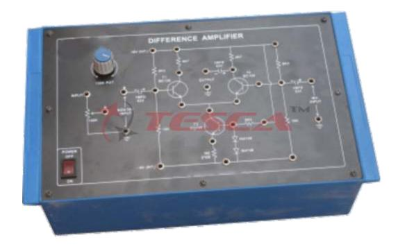
Experimental Training Board has been designed specifically for the study of Differential Amplifier in solid state version. A Differential Amplifier is also called a Differential Amplifier and it is essential part of operational amplifier. As operational amplifiers are now a days being used quite extensively in instru-mentation control and entertainment electronics, this Training Board has great educational value.
