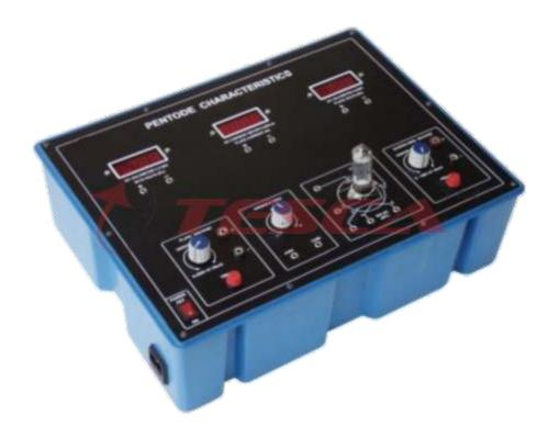
Experimental Training Board has been designed specifically to study the characteristics of a Pentode. The board is absolutely self contained and requires no other apparatus.
