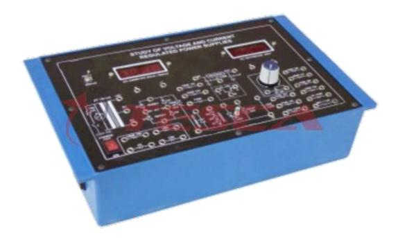
Experimental Training Board has been designed specifically for the study of difference between Voltage Regulated and Current Regulated Power Supplies. Certain basic circuits used in such supplies can be assembled and studied on this training board. The board is absolutely self contained and requires no other apparatus.
