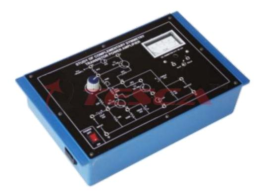
Experimental Training Board has been designed specifically for the study of Complementary Symmetry Transistor Power Amplifier. This training board is quite useful for measuring D.C. bias current and observation of waveforms.
