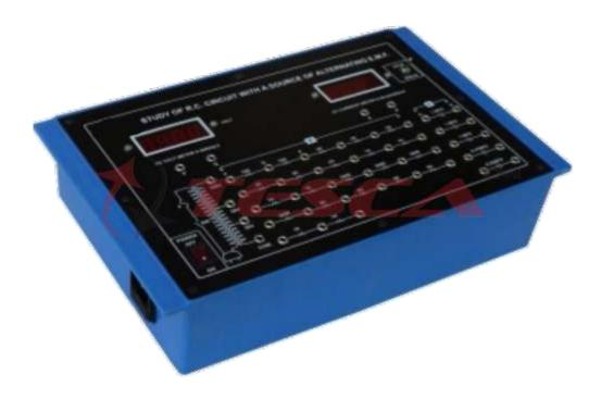
Experimental Training Board has been designed specifically for the study of R-C Circuit with a Source of Alternating E.M.F. The board is absolutely self contained and requires no other apparatus.
