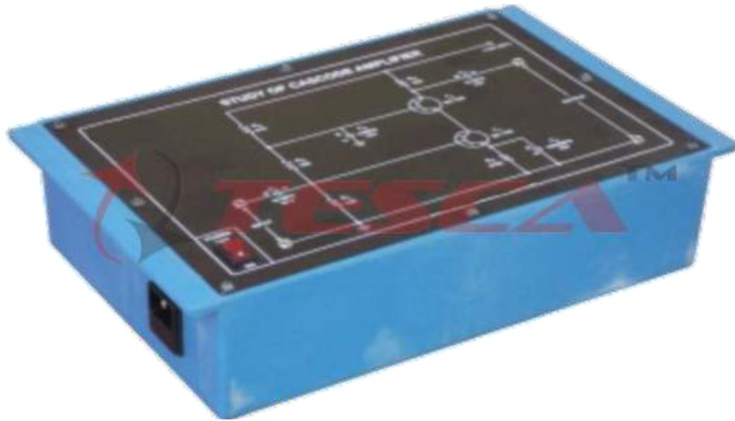
Experimental Training Board has been designed specifically for the study of Cascode Amplifier. Various parameters of a Cascode Amplifier can be measured on this training board.
