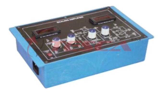
Experimental Training Board has been designed specifically for the study of Scaling Amplifier using OP-AMP Ics 741. The board is absolutely self-contained and requires no other apparatus.
