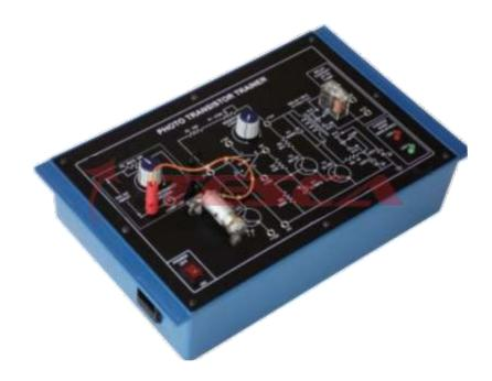
Experimental Training Board has been designed specifically for the Study of Photo Transistor and its Application.
