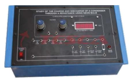
Experimental Training Board has been designed specifically to study the Charge and Discharge of a condenser through a resistance using neon bulb.
