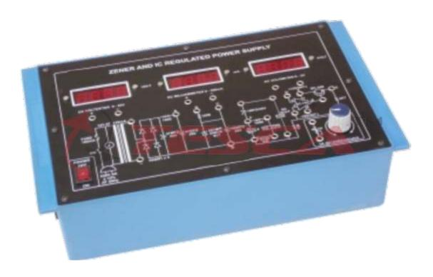
Experimental Training Board has been designed specifically for the study of zener regulated and IC regulated power supply. This training board is absolutely self contained and requires no other apparatus.
