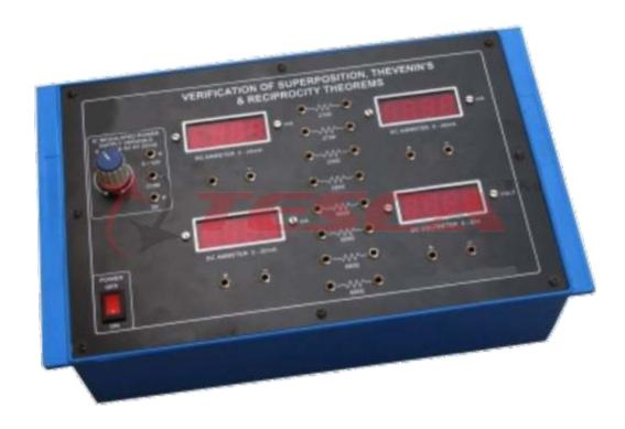
Experimental training board has been designed specifically for the study & verification of network theorems in D.C. circuits. The board is absolutely self-contained and requires no other apparatus.
