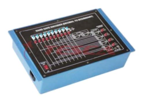
Computer Logic Training Board has been designed specifically for the study of NAND gate Encoder, to encode Decimal number to BCD(binary coded) equivalent. This Training Board gives a better understanding of the phenomena of encoder using four input NAND gates with ten decimal inputs and 4-bit binary output. The board is absolutely self contained and requires no other apparatus.
