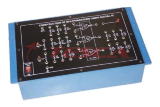
Computer Logic Training Board has been designed specifically for the study of Bistable, Monostable & Astable multivibrators using digital IC. This Training Board gives a better understanding of the concepts involved in construction of multivibrators and their properties. The board is absolutely self-contained and requires no other apparatus.
