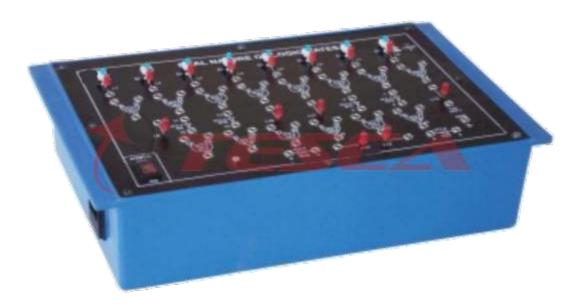
Computer Logic Training Board has been designed specifically for the study of Dual Nature of Logic Gates. This Training Board gives a better understanding of the phenomena of duality with the help of verification of truth tables of Dual gates. This board also explains combinational logic function Boolean variables and generation of truth tables.
