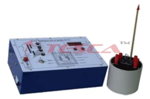
**55763** Experimental Set Up has been designed specifically for determination of Curie Temperature of Monel Metal using a Transformer. The set-up consists of Monel Metal Transformer, Container, Heater, Thermometer, Stirrer etc. The set up is complete in all respect and requires no other apparatus. Practical experience on this set up carries great educative value for Science and Engineering Students.
