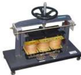
Three Phase Inductive Load
