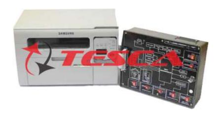
10950 trainer is a very versatile training system, has been designed to explain 3 in 1 Laser Printer hardware and its trouble shooting. Various test points have been provided so that one can check inputs and outputs of each block contained. Being different from a conventional block diagram internal structure of blocks is also shown. Test points allow the analysis and monitoring of the signals in different sections.
