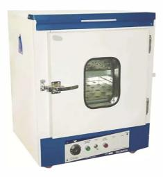
Double walled, Outer made of GI/MS Powder Coated. Element of three sides' SS Chamber Digitally controlled Temp. Range 5°C above RT to  $70^{\circ}$ C,  $\pm$  0.5°C, fitted with fan & Digital Electronic Timer 99.99 Hours having double viewing window, supplied with shelves workable on 220/230 volts A.C.
