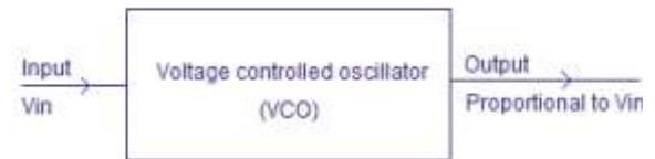
Block Diagram of Voltage Controlled Oscillator
