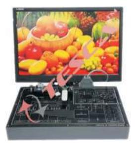
10944A is a LCD/LED Colour TV Trainer is an ideal training equipment to teach the operation of LCD/LED colour TV receivers. The complete Block of LCD/LED TV Receiver is printed on single PCB for easy understanding of function of different blocks. Test points allow the analysis and monitoring of the signals in different sections. By using the fault simulation method, it is possible to introduce the most common breakdown and their rectification.
