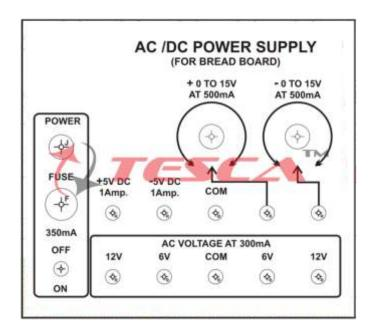
**16949** AC DC POWER SUPPLY has been designed specifically for Electrical /Electronics Lab where fixed DC +5Volt At 1Amp, Fixed DC-5V At 1Amp, Variable 0 - 15 V DC at 500mA & 0 to -15V DC At 500mA . AC voltage 0-6-12-18-24 Volt At 300mA or AC Voltage 12V-6V-0V-6V-12V at 300mA.
