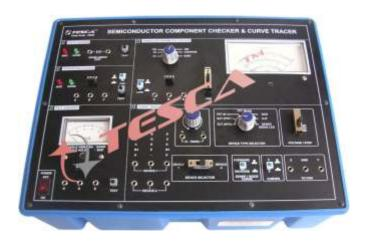
$16950 \ \ Semiconductor \ component \ checker \ \& \ curve \ tracer \ are \ useful \ for \ checking \ \& \ tracing \ the \ characteristics \ curve \ of \ a \ variety \ of \ components \ in \ a \ very \ short \ time \ duration. \ The \ Instrument \ consist \ of \ five \ different \ sections, \ detail \ Specifications \ \& \ features \ are \ following:$
