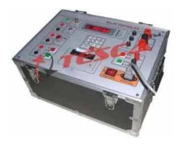
19557 is an ideal, newly developed multifunction relay tester adopting monolithic computer technology. It is composed of auto synchronized digital millisecond timer, logic controlling unit, multifunction digital display, high precision digit collection and processing unit, current-voltage output unit, overload and over range protection unit. Test process is automatic for improved efficiency. The tester has a built in printer for printing the results.
