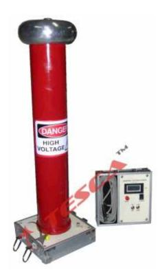
19562 is high voltage divider and digital meter. The top terminal of the voltage divider is connected to high voltage output under test / calibration. The voltage divider is connected to digital meter by measuring cable provided.
