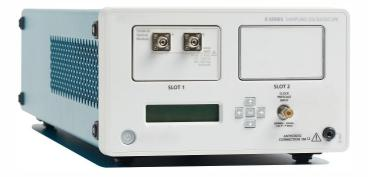
Sampling Oscilloscope provides a comprehensive optical test solution for telecom and datacom applications, as well as general purpose optical component testing. The sampling oscilloscope optical modules provide > 30 GHz optical bandwidth, plus fully integrated Optical Reference Receivers (ORR)1 enabling both single mode and multimode conformance testing at 850 nm, 1310 nm, and 1550 nm bands.
