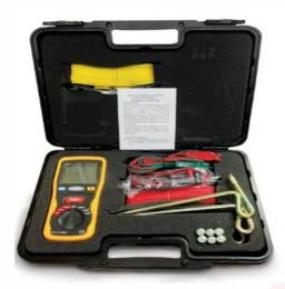
Electronic Digital Earth Resistance Tester is direct replacement of the conventional hand generator type tester. It is designed for measurement of the resistance of earthing used in the electrical equipment as well as for measurement of ground resistivity. It can be used for measurements of the other low regular and liquid resistances. It can also be used for measurement of voltage AC, voltage DC and resistance.
