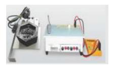
• Force / Weight : measurement using piezo transducer (0- 20 kg) weighing scale sensor
