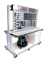
Double-Sided Mobile Workstation Allows The Assembly And Operation Of The Various Components Without The Use Of Tools (components Equipped With Quick Assembly System) The Workstation Must Be Equipped With: Pneumatic Basic Working Table (double Side):
