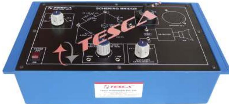
Experimental Training Board has been designed specifically to Measure the Value of unknown Capacitance by Schering Bridge.
