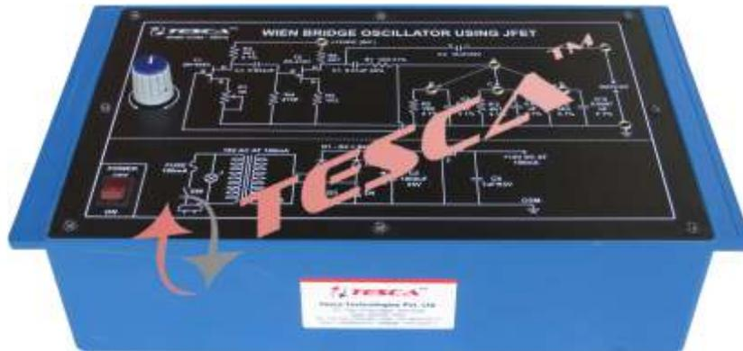
The experimental set up has been designed specially for the study of Wien Bridge Audio Oscillator using JFET. The Training board helps us to understand the utilization of Audio OSC and obtain oscillation at different frequencies.
