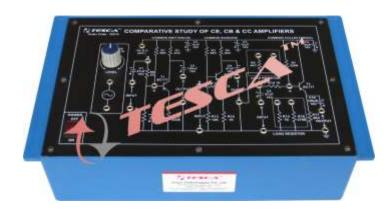
Experimental Training Board has been designed specifically for the Comparative study of Common Emitter (CE), Common Base (CB) and Common Collector (CC) Transistor Amplifiers. These practical transistor amplifier configurations are evaluated in respect of their main parameters and results are compared with theoretical calculations.
