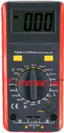
A LCR meter (Inductance (L), Capacitance (C), and Resistance) is a piece of electronic test equipment used to measure the inductance, capacitance and, resistance of a component. In the usual versions of this instrument these quantities are not measured directly, but determined from a measurement of impedance.
