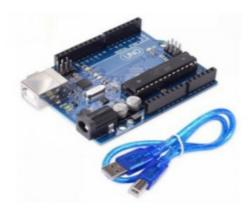
**Description-** The Arduino Uno R3 with Cable is a microcontroller board based on the ATmega328 (datasheet). It has 14 digital input/output pins (of which 6 can be used as PWM outputs); 6 analog inputs, a 16 MHz ceramic resonator, a USB connection, a power jack, an ICSP header, and a reset button.
