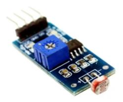
**Description-**This LM393 Photosensitive Light-Dependent Control Sensor LDR Module is using a high-quality LM393 voltage comparator. Easy to install using the sensitive type photosensitive resistance sensor the comparator output signal gives a clean and good waveform.
