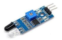
**Description-** IR Infrared Obstacle Avoidance Sensor Module has a pair of infrared transmitting and receiving tubes. When the transmitted light waves are reflected back, the reflected IR waves will be received by the receiver tube. The onboard comparator circuitry does the processing and the green indicator LED comes to life.
