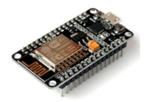
**Description-**The ESP8266 NodeMCU CP2102 board has ESP8266 which is a highly integrated chip designed for the needs of a new connected world. It offers a complete and self-contained Wi-Fi networking solution, allowing it to either host the application or to offload all Wi-Fi networking functions from another application processor.
