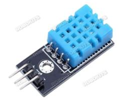
**Description-** This module integrates DHT11 sensor and other required components on a small PCB. The DHT11 sensor includes a resistive-type humidity measurement component, an NTC temperature measurement component and a high-performance 8-bit microcontroller inside, and provides calibrated digital signal output.
