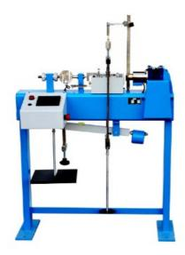
**Application:** Apparatus should be used to test resisting shear strength of soil specimen.
