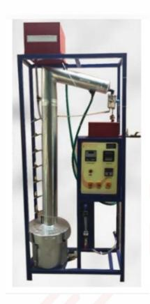
Description:- The Set Up Consists Of A Column Fitted With Perforated Plates. Liquid Is Fed At The Top Of The Column Through Distributor. The Solute Gas And Air Are Measured Separately, Mixed In A Mixing Chamber And Then Passed Through The Perforated Plates Vertically Upward And Absorbed In Liquid. All The Flow Rates Can Be Independently Varied To Simulate Different Conditions. Liquid Sample Can Be Taken Out From The Bottom Of The Column For Analysis.
