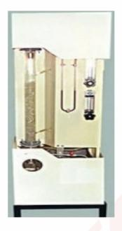
**Description:-** The Set Up Is Capable Of Studying The Loading And Flooding Characteristics. It Is A Packed Column Packed With Rasching Rings Where The Air Is Counter Currently Fed To The Column. The Liquid Holdup In The Column Increases The Weight Of Column And Also Reduces The Effective Porosity Of Packing. This Reduction In Porosity Decreases The Gas Velocity, Increases The Pressure Drop And Changes The Value Of Mass Transfer Coefficient.
