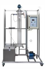
**Introduction:** This Instrument Is Used To Investigate Basic Hydrostatic Principles, Installation And Calibration And Maintenance Of The Process Using A Column Of Water. The Device Includes A Clear Acrylic Tank And A Feed Tank. Tools Of Different Design And Manufacture Can Be Installed By Means Of Quick Couplings Placed On The Device And On The Tank. Differential Pressure Transmitter Is Included This Instrument Offers Training Programs
